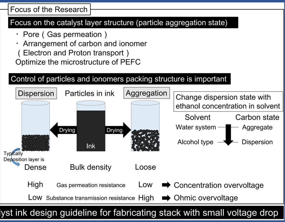
**Aim of the Research** ) Establishment of optimal catalyst ink design guideline for fabricating stack with small voltage drop
